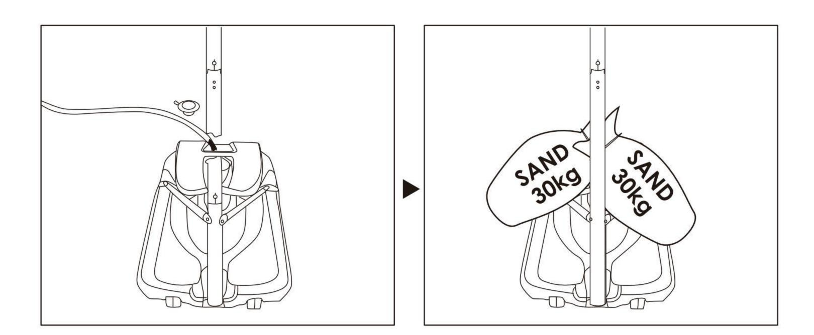
The base can be filled with either water or sand, but for your convenience and stability of the basketball hoop, we suggest filling it with water and adding a sandbag on top of the water-filled base.
