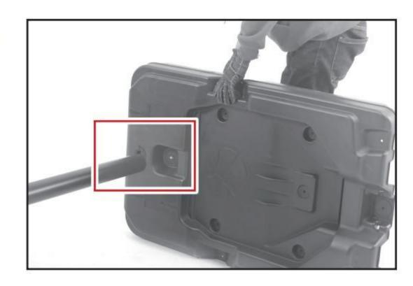
Apply the long pole braces (U1) and short pole braces (U2) to the base using provided 4 M8×20 mm screws, 8 washers, and 4 locknuts.
