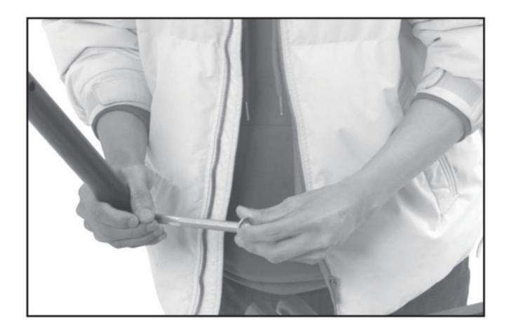
2. Fix the two short backboard braces to the bracket using 2 M12 washers and a nut through the Ø16×70 mm bushing as shown.
