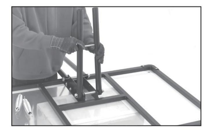
5. Hook the ends of the big springs onto the bracket and the other ends on the M10 bolt as shown.
