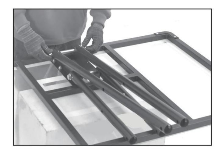
Pass the M10×160 mm bolt through the middle holes of the two short backboard braces, and use an M10 nut to lock it.
