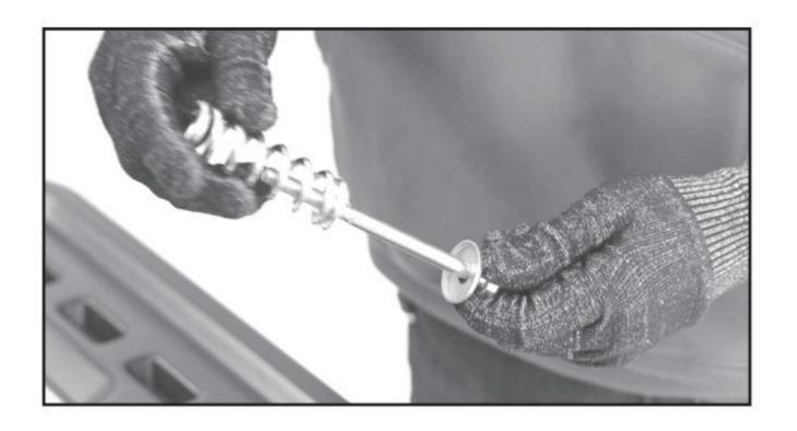
Insert them into the remaining 2 holes on the rim from the rim side of the backboard and tighten them using 2 M8 nuts.
