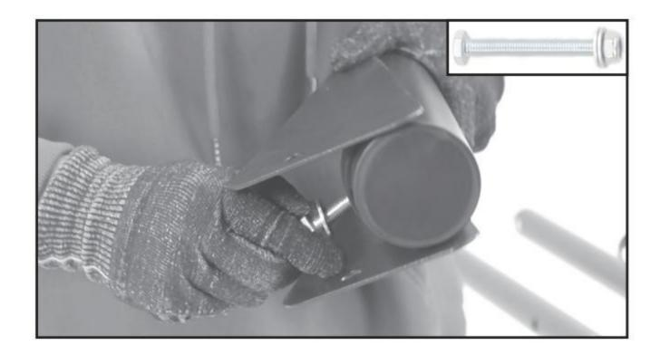
Attach the upper rod to the backboard braces using 2 M12×160 mm bolts, 8 M12 washers, and 2 nuts.
